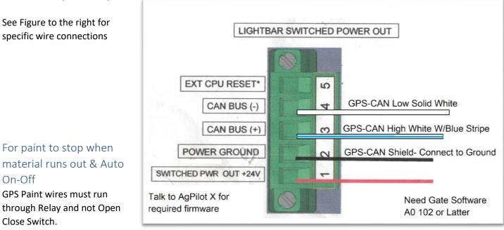
To install and have GPS Paint signal work in auto mode, See image below.
